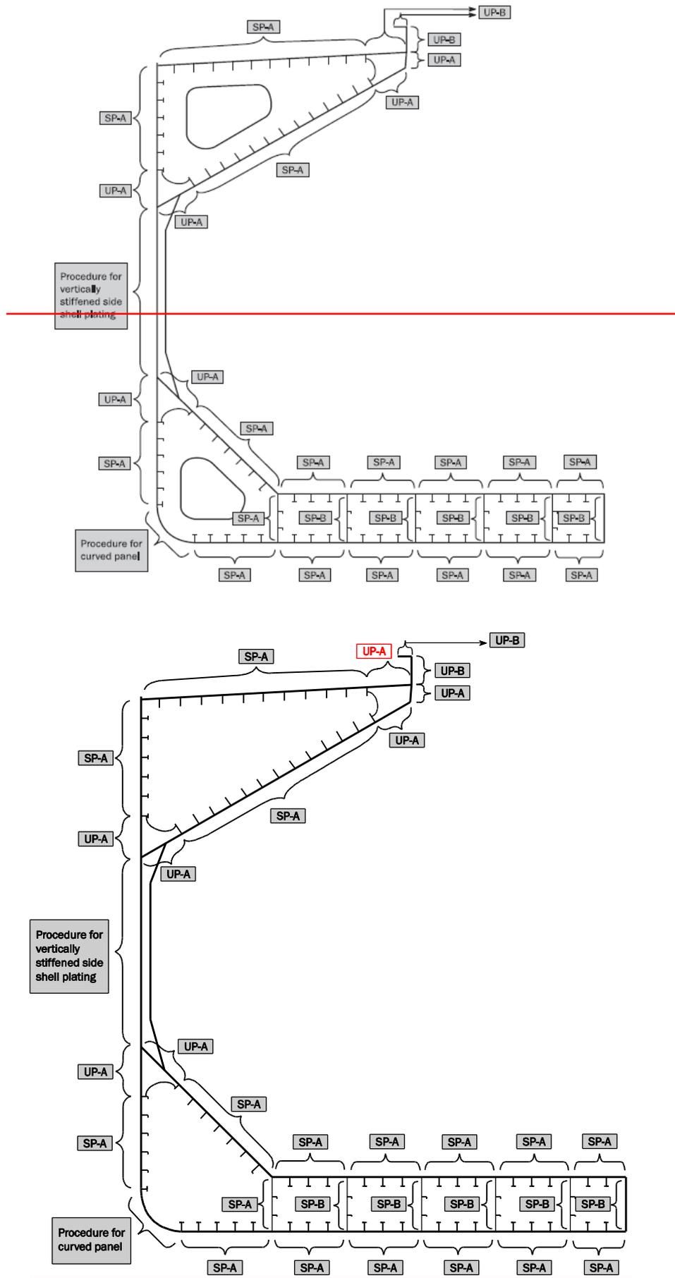
Figure 7 : Longitudinal plates for double hull bulk carrier
