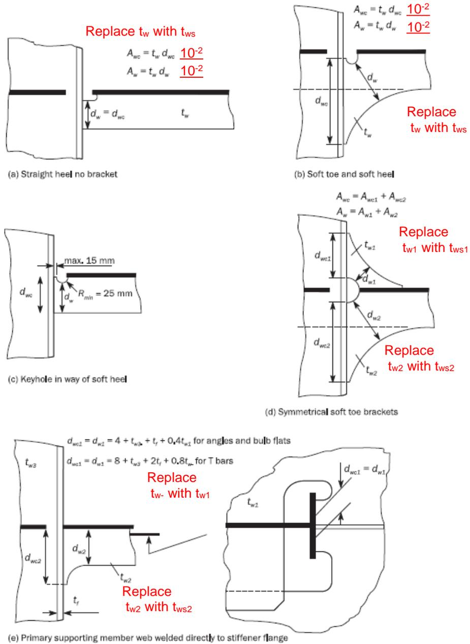
$t_{ws}$ ,  $t_{ws1}$ ,  $t_{ws2}$ : Net thickness of the primary supporting member web stiffener/backing bracket, in mm.
